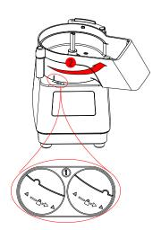
• Mount the ejector flat on the drive shaft.
