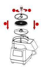
• Tips: To cut products of different hardness with an grid, start by cutting the soft products first, as these cannot push the diced hard product trapped in the grid. For hard products such as carrots, celery, we advise using the round hopper.
